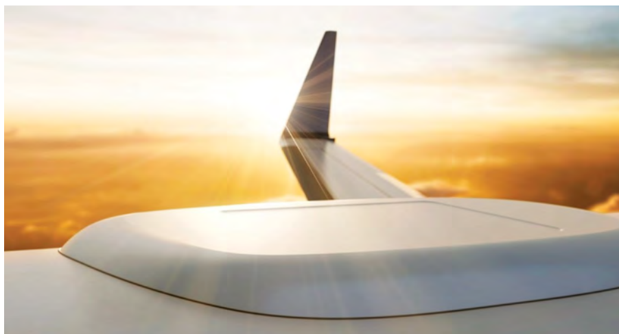
Project Kuiper's aviation-specific customer terminal is based on Amazon's most powerful Kuiper terminal—a full-duplex, Ka-band phased array antenna that can support download speeds up to 1 Gbps on a single device. (Copyright/Credit: Amazon.)
