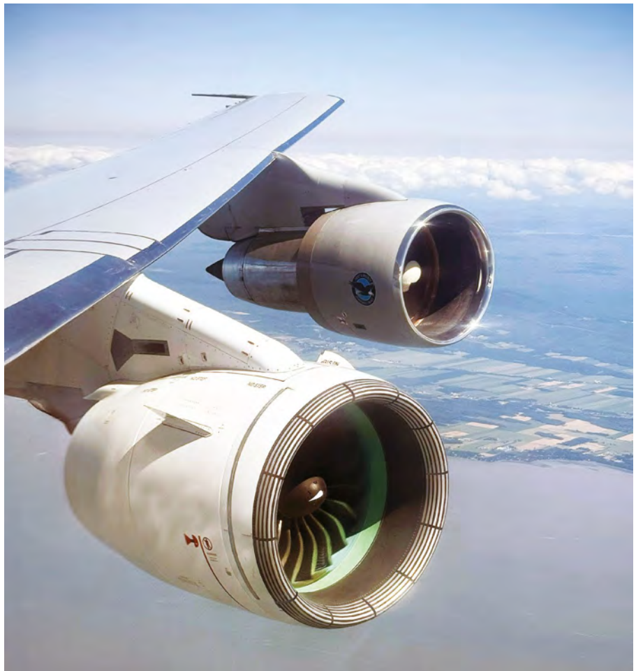
Certification flight testing for the GTF Hot Section Plus is underway on Pratt & Whitney's 747 flying test bed in Mirabel, Canada. (Copyright/Credit: Pratt & Whitney.)
