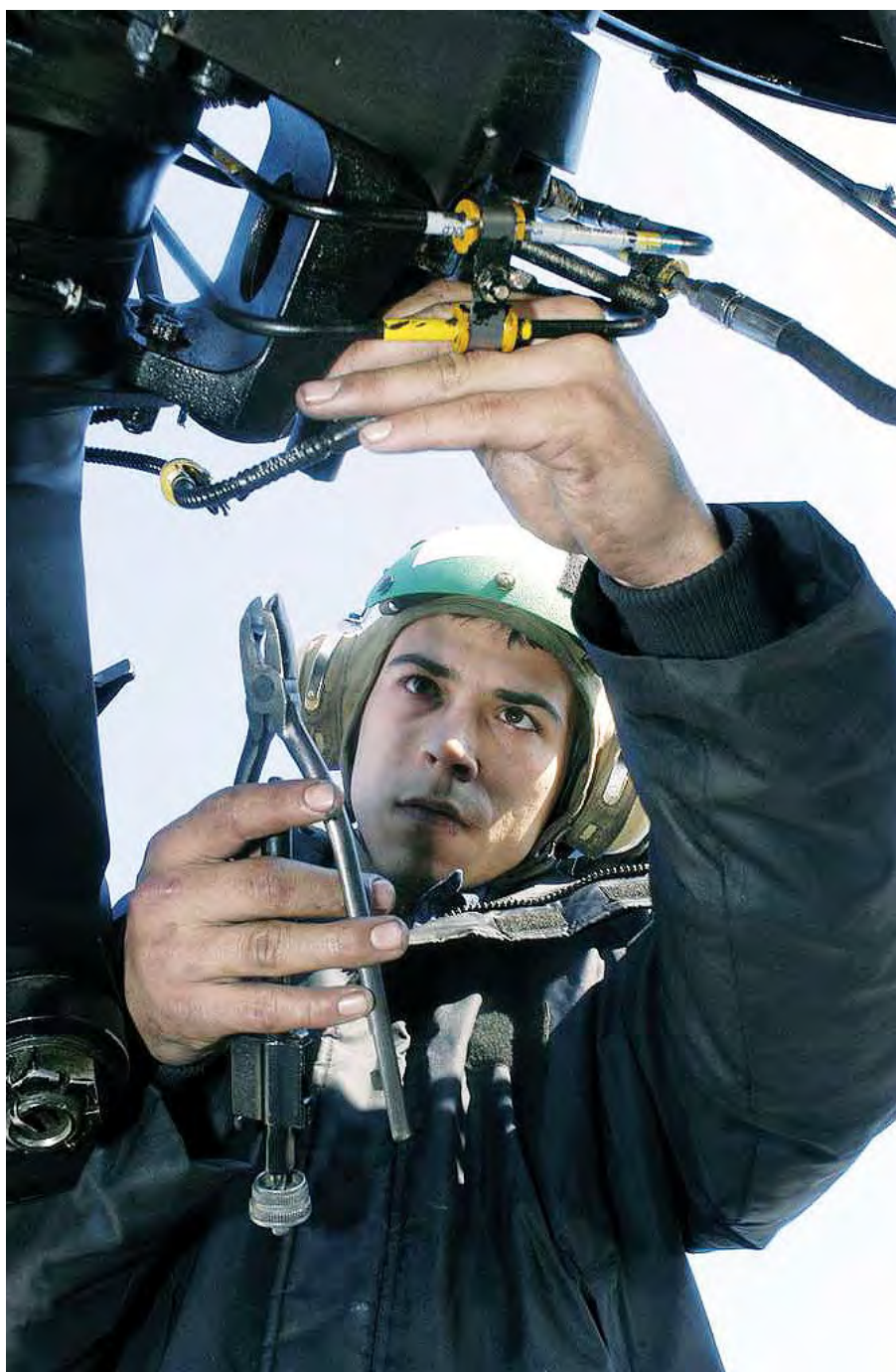
An aviation electrician replaces a blade wire harness on an MH-53E Sea Dragon. (Copyright: Picryl.)
