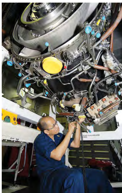
An aviation machinist installs a wiring harness on an F-A-18E Super Hornet engine. (Copyright: Picryl.)
