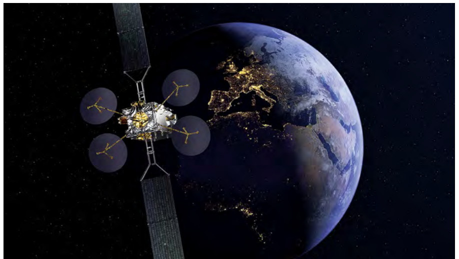
On launch, EUTELSAT KONNECT VHTS, was the largest GEO satellite to date in Europe, delivering 230 beams and with a Ka-band capacity of 500Gbps. (Copyright/Credit: Thales Alenia Space.)
