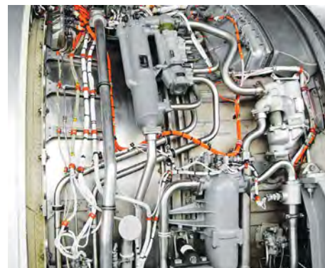
Wires and pipes outside the lining of an airplane's turbine engine. (Copyright: Cloom Tech.)
