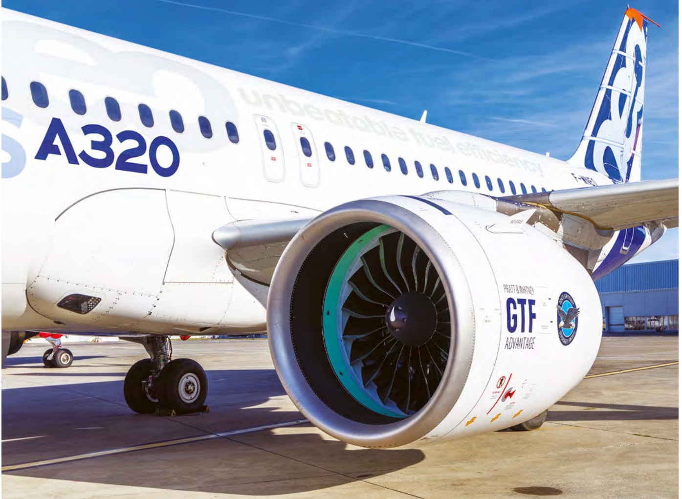
The Pratt & Whitney GTF Advantage engine powering the Airbus A320neo Family aircraft. (Copyright/Credit: Airbus.)
