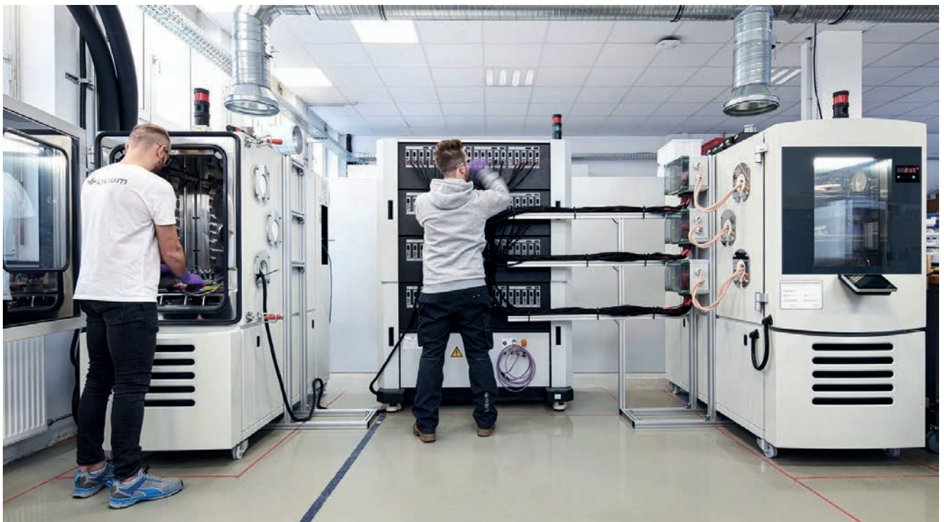
The Lilium team testing cells against its mission profile at its HQ near Munich. (Copyright: Lilium)
