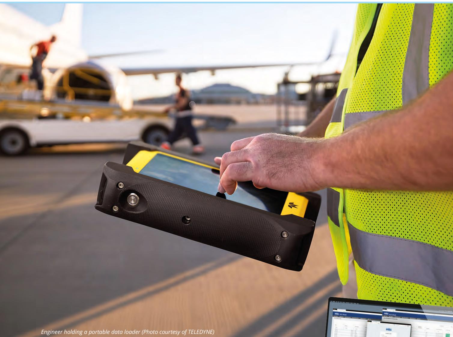
Engineer holding a portable data loader (Photo courtesy of TELEDYNE)
