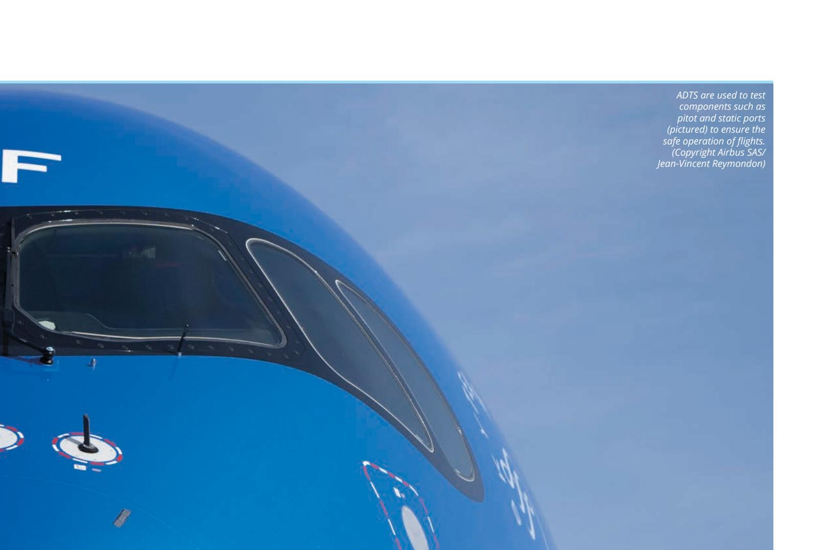
*ADTS are used to test components such as pitot and static ports (pictured) to ensure the safe operation of flights. (Copyright Airbus SAS/ Jean-Vincent Reymondon)*
