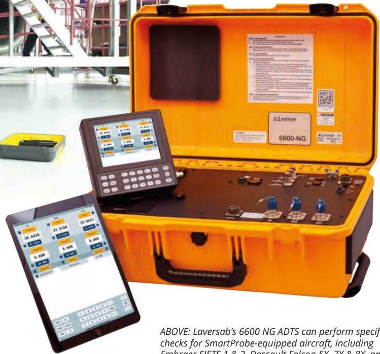
ABOVE: Laversab's 6600 NG ADTS can perform specific checks for SmartProbe-equipped aircraft, including Embraer EJET 1 & 2, Dassault Falcon 5X, 7X & 8X, and the Gulfstream G650. (Copyright Laversab)
