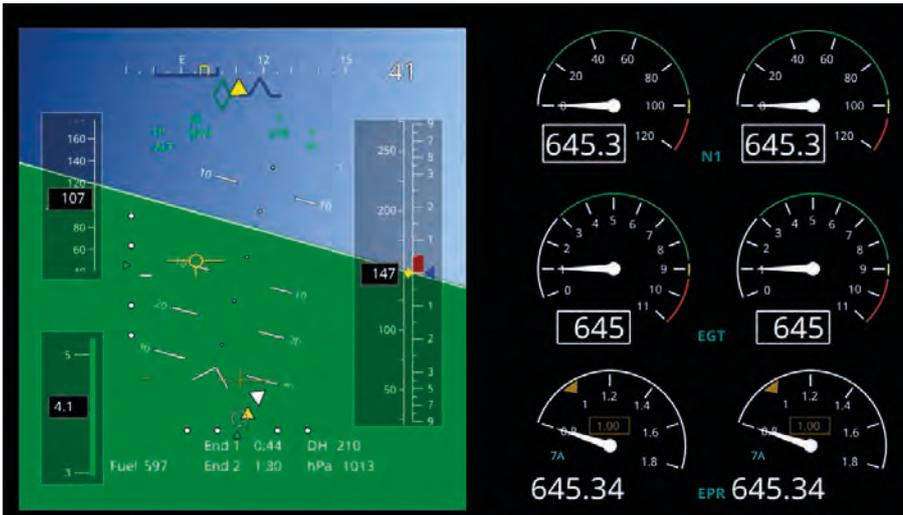
Shared Screen Example with PFD and Engine Subsystem on Same Display
