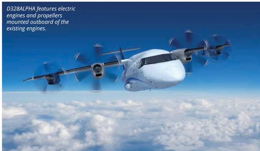
*D328ALPHA features electric engines and propellers mounted outboard of the existing engines.*
