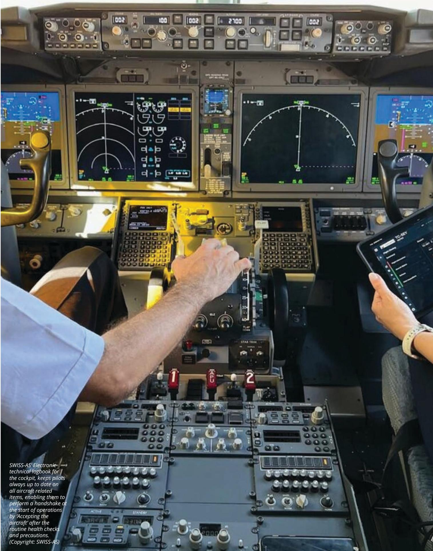
SWISS-AS' Electronic technical logbook for the cockpit, keeps pilots always up to date on all aircraft related items, enabling them to perform a handshake at the start of operations by 'Accepting the aircraft' after the routine health checks and precautions. (Copyright: SWISS-AS)
