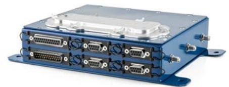
Bottom Image: AFIRS Edge serves as an Internet of Things (IoT) gateway on the aircraft ready to support new IoT sensor technologies as they are deployed. (Copyright: FLYHT)
